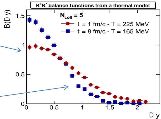
Model prediction ( $\sigma_{\eta}=0$ ) of the Charge Balancing Width in the  $\eta$  direction
